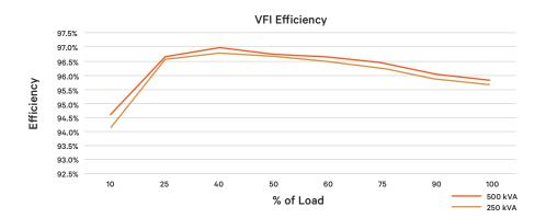
The new generation architecture of Liebert® APM Plus has been designed to reduce energy and heat dissipation, consequently minimizing the demand and consumption of air conditioning systems.
